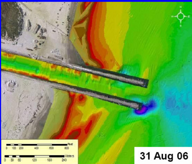
Summer – Scour at mouth radiates from south jetty
